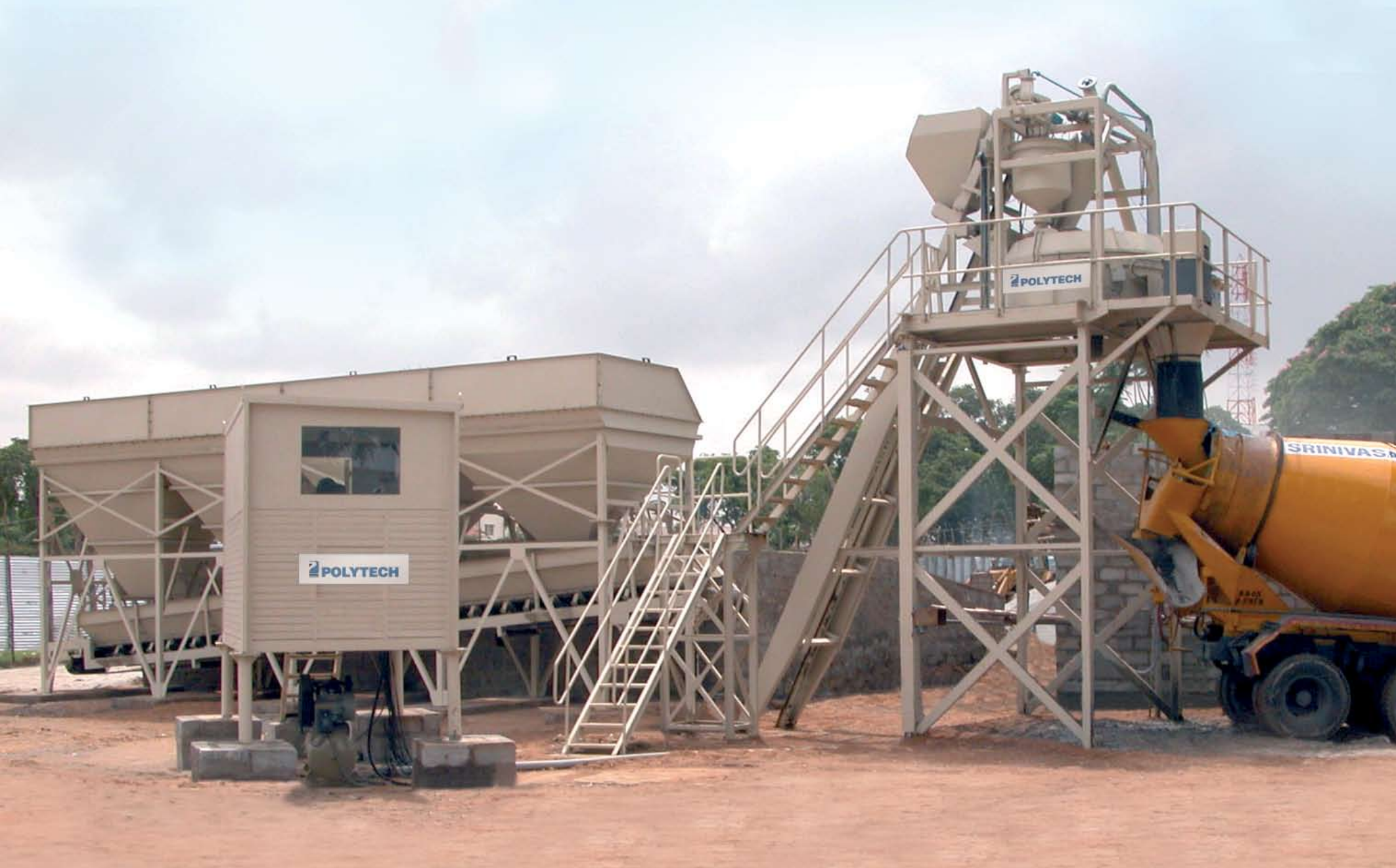
Plant installation at ISKCON project site, Bangalore Capacity: 30 M 3 /Hr. Srinivasa RMC, Bangalore
